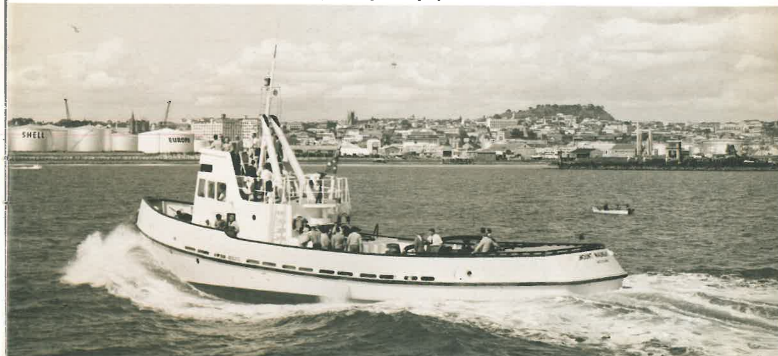
BELOW: The tug 'Mount Maunganui' , designed and constructed by Mason Bros, was the first vessel built in New Zealand to Lloyd's stringent A1 specification.
