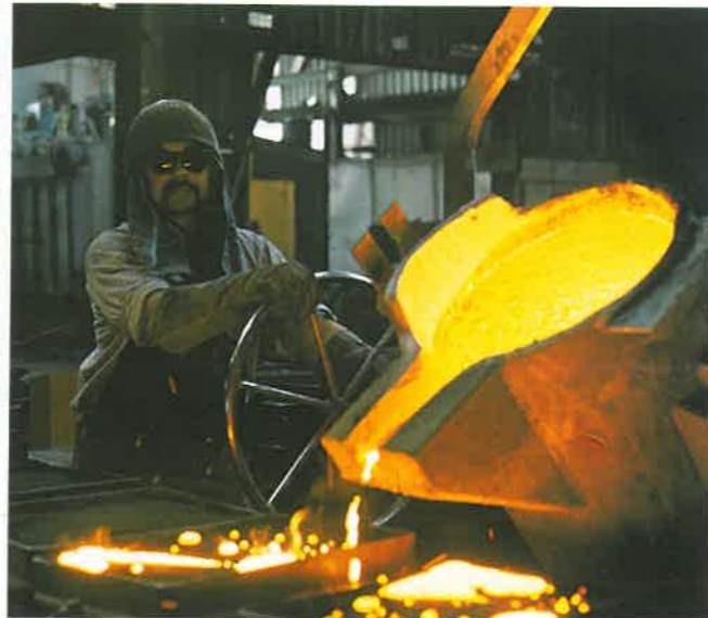
ABOVE: Caster Sam Tasse directs molten metal from a ladle into moulds at the Christchurch plant of Andersons Foundry Ltd, producer of castings in a variety of irons for applications in industry throughout New Zealand.
