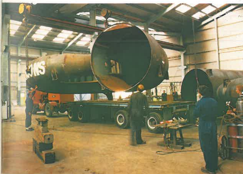
BELOW: Heavy engineering and steel fabrication is performed by subsidiary companies at Palmerston North, Auckland and Christchurch. Shown is part of the large workshops of Andersons Engineering Ltd, Christchurch, where scroll casings for a North Island hydro-electric development are being despatched.
