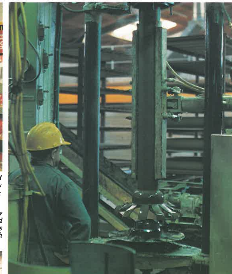
ABOVE: Automatic machinery is used to produce ceramic pipes and fittings at A.B. Pipes Ltd in metropolitan Auckland. In contrast, the company's Carterton works, located in the heart of the rural region it serves (below), employs traditional methods to produce drainage pipes and tiles.
