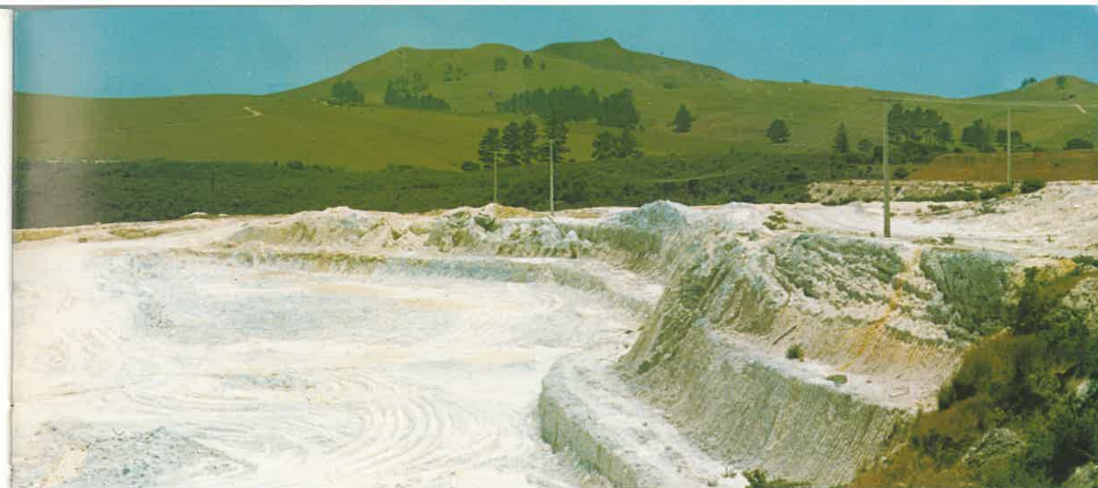
ABOVE: Stark white in evidence of its low contaminant level, this deposit of china clay at Matauri Bay, north of Auckland, is worked by New Zealand China Clays Ltd, which also processes the material, principally for export to crockery and paper manufacturers.
