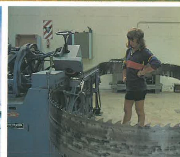
ABOVE: Sawmilling equipment, like this bandsaw sharpening machine at The Fletcher Timber Company's new mill at Kopu, near Thames, is part of a range of merchandise supplied by Charles Palmer & Company.
